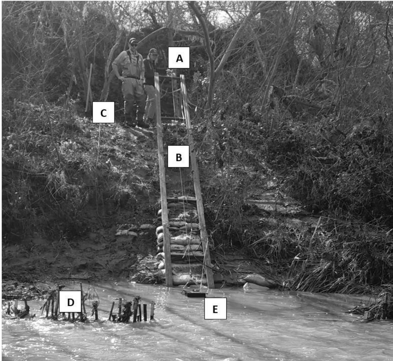
Figure 2. Salsipuedes Creek DIDSON monitoring site in 2019 with key features labeled. (A) winch; (B) track; (C) cross-bracing cables; (D) deflection panels; (E) DIDSON/X2/sled assembly.
